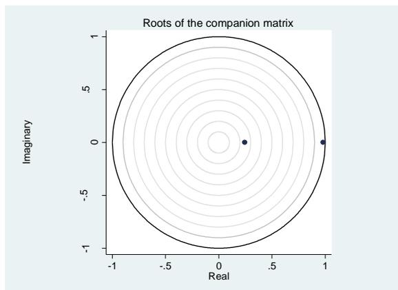
**Figure 1: Eigenvalue stability condition**
